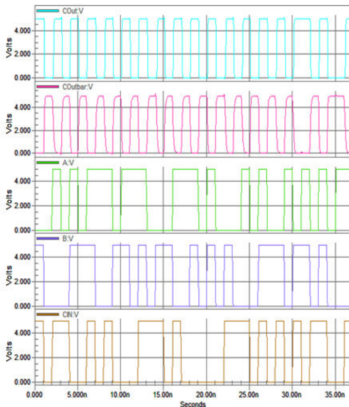
Figure.3 Delays for carry outputs
