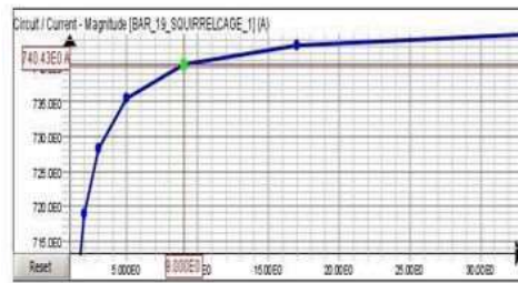
Fig22: Current response in rotor bar no:19
