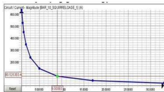
Fig17: Current response in rotor bar no:10
