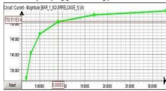
Fig20: Current response in rotor bar no:11
