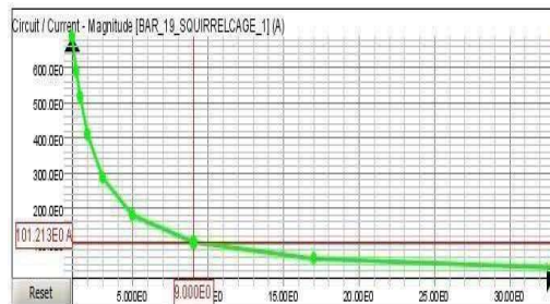
Fig11: current response in rotor barno:19
