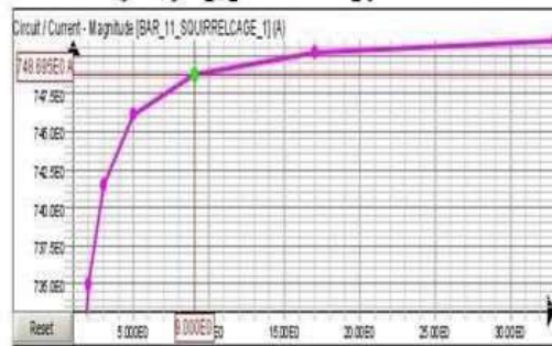
Fig21: Current response in rotor bar no:1
