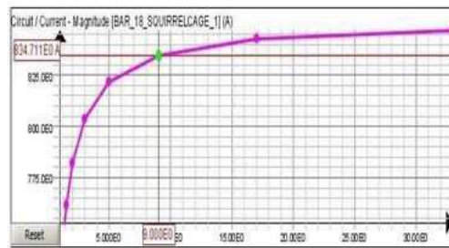
Fig:14 Current response in rotor bar no:18
